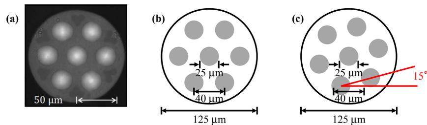
Fig. 2. Cross-sections: (a) multimode multicore fiber © [2012] IEEE. Reprinted, with permission, from [10], (b) fan-in/out polymer waveguide designed to connect with (a), and (c) 15° tilted structure of (b).
