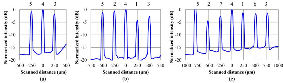
Fig. 15. Output power profile at one-dimensionally aligned core end of (A) 3-core fan-in/out waveguide, (B) 5-core waveguide, and (C) 7-core waveguide.
