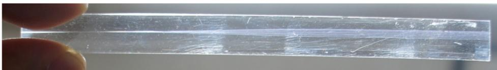
Fig. 14. Over-view of a fabricated 7-core fan-in/out waveguide.
