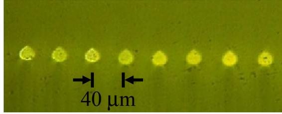
Fig. 3. Cross-section of a fabricated waveguide with 25- $\mu\text{m}$  core diameter and 40- $\mu\text{m}$  interchannel pitch.
