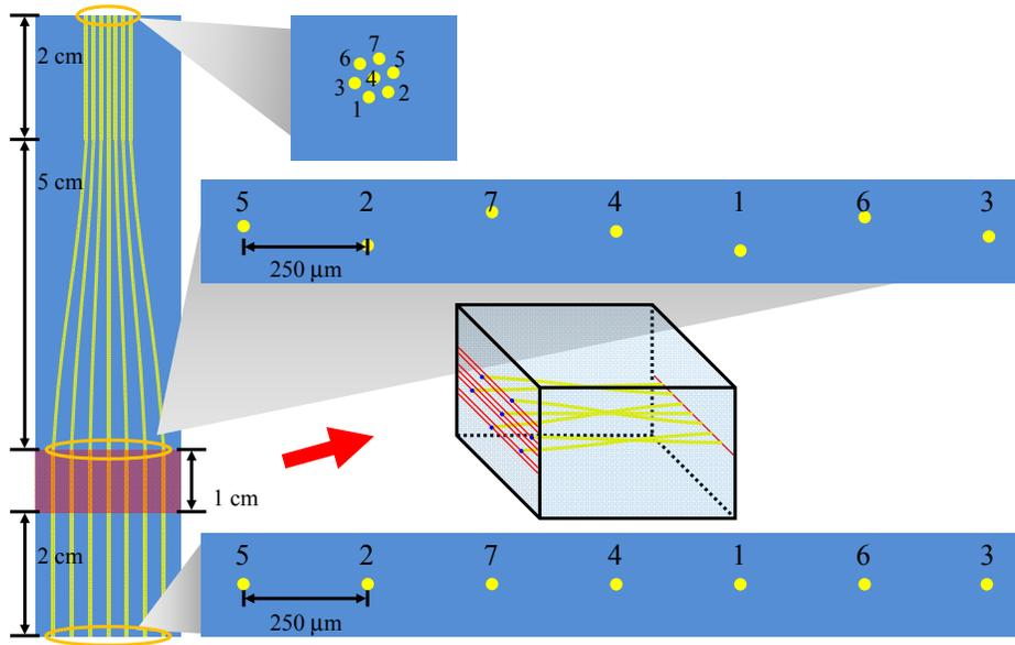
Fig. 4. Fan-in/out waveguide design.
