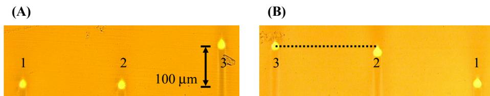
Fig. 8. Cross-sections of a fabricated vertical bending waveguide.
