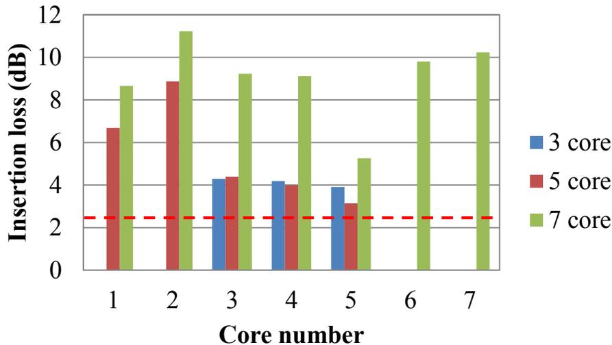
Fig. 16. Insertion loss of the fabricated 3-core, 5-core, and 7-core fan-in/out waveguides at 850-nm wavelength (10-cm long). Red broken line: Averaged insertion loss of 10-cm long straight waveguide.
